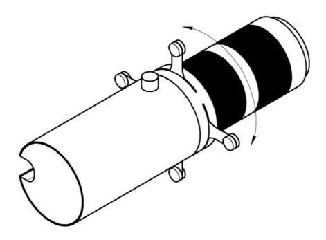
5. The telescopic mechanism of the lens system adjusts the projection angle from 20° to 35° by zooming in/out built-in condenser lenses (ZOOM). Attention! See p. 3.
