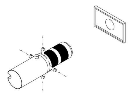
2. A special device for installing color light filters or a plate (gobo) with a stencil of logos and various patterns;
